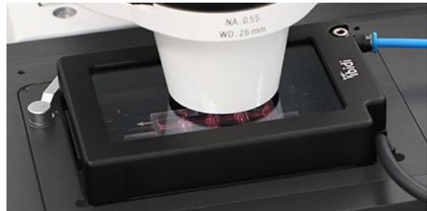
During a live cell imaging experiment, the evaporation in the stage top incubator should be kept as low as possible, underlining the need for a reliable humidity control. A constant and high level of humidity (>90% RH) in the stage top incubator is one of the keys to artifact-free results in live cell imaging.
