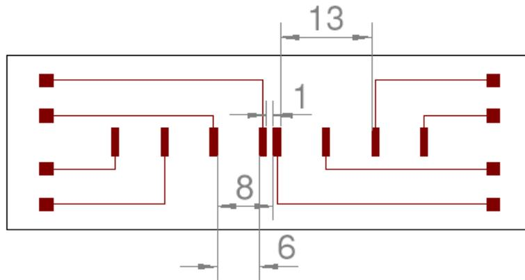
Fig 2: electrode slide with distances of the electrodes. The electrodes are 1 mm wide
