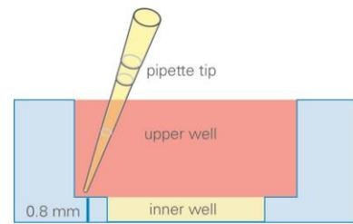
**Figure 3: Using the pipette in one well of the  $\mu$ -Slide Angiogenesis.**
