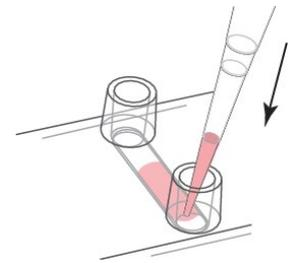
*Filling in a cell suspension into one channel of the  $\mu$ -Slide VI<sup>0.4</sup>.*
