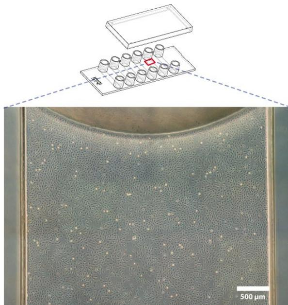
Unlike in open wells, the channel does not disturb the beam path of the phase contrast microscope.
