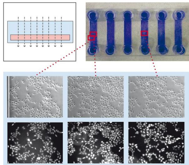
*Geometric scheme and cell distribution in the  $\mu$ -Slide 8 Well (left) and the  $\mu$ -Slide VI<sup>0.4</sup> (right). Please note the typical non-homogeneous cell distribution in an open well caused by the natural meniscus effect and handling of the slide. Cells were visualized macroscopically using crystal violet staining (top), and microscopically using phase contrast (middle) and fluorescence microscopy (bottom).*
