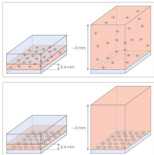
*When using the  $\mu$ -Slide VI<sup>0.4</sup> (left) and the  $\mu$ -Slide 8 Well<sup>high</sup> (right), different cell concentrations must be seeded to get the same number of adherent cells per unit area. The example shown here is with 25 cells.*
