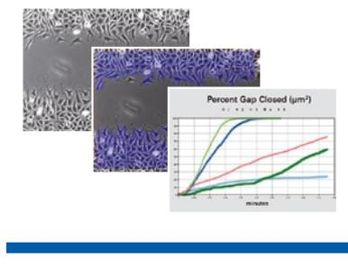
The [ibidi Culture-Inserts with 2 Wells, 3 Wells, or 4 Wells](#) are silicone inserts with a defined cell-free gap for wound healing, migration, 2D invasion assays, and co-cultivation of cells. They are available as individual inserts in a  $\mu$ -Dish or as 25 pieces for self-insertion. For high-throughput experiments, we provide the [Culture-Insert 2 Well 24](#).
