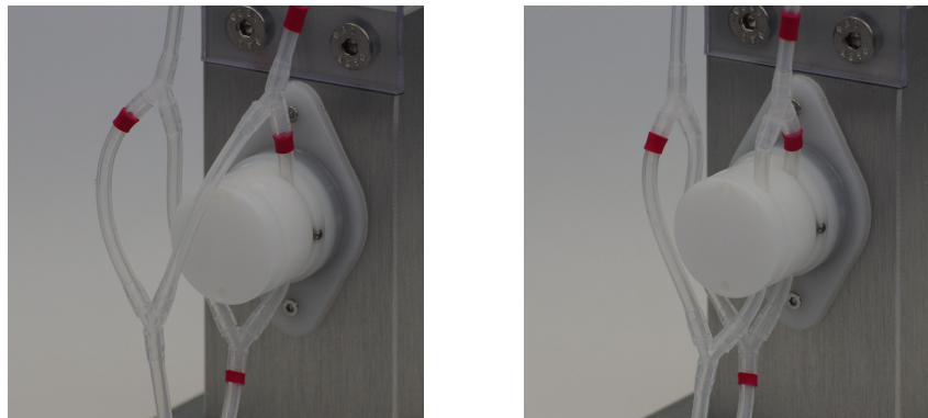
Figure 23: Insert the tubing coming from reservoir B into the right side slots. The marked tubing goes in the rear slot.
