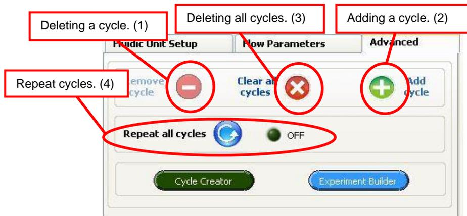
Figure 11: Adding and deleting cycles.
