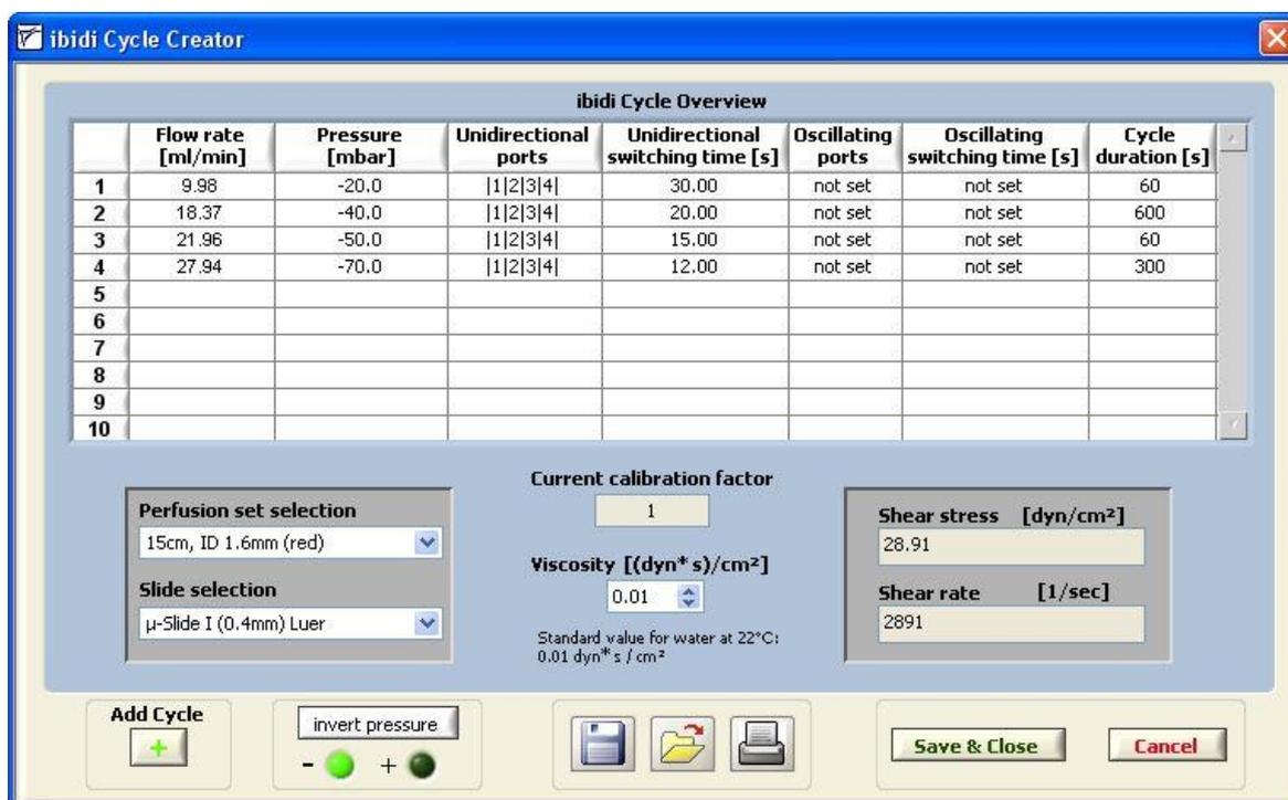
Figure 16: Set of cycles in the 'Cycle Creator' table.
