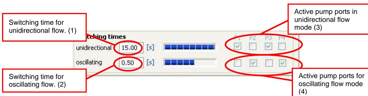
Figure 10: Switching times and active pump ports.
