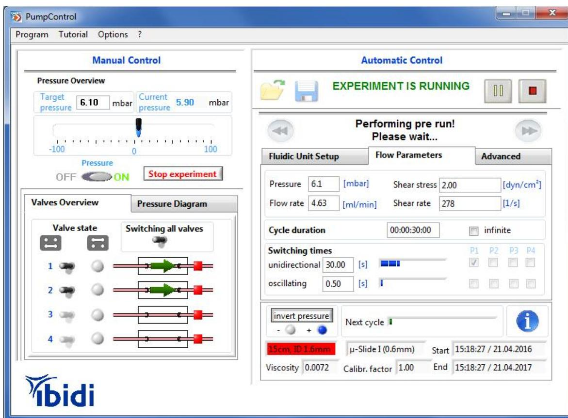
The automatic control was developed to perform exact cycles over seconds, minutes, days, or even weeks. With this tool, the shear stress, which is applied to the cells in the  $\mu$ -Slide, can either be set by choosing the air pressure, the flow rate, or the shear rate, or by directly entering the shear stress. In any of these cases, the program will automatically calculate the
