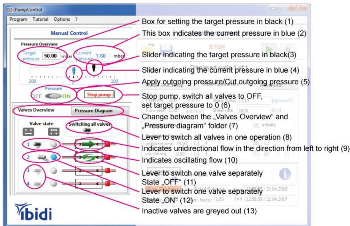
Figure 4: Manual control of the ibidi Pump with the control buttons on the left of the PumpControl software window.
