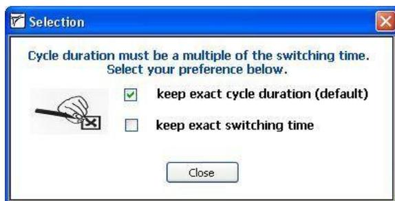
The default setting keeps the exact cycle duration. This option will adjust the switching time. The other setting keeps the exact switching time. When you choose this option, the cycle duration will be adjusted.
