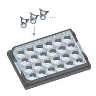
2. Switch to the culture position where the inserts are lifted 1 mm above the coverslip by carefully pushing the frame to the left.
