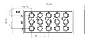
Every well of the  $\mu$ -Slide 15 Well 3D Glass Bottom consists of an inner and an upper well. This "well-in-a-well" technology reduces gel volumes to 10  $\mu$ l per well, and no gel meniscus is formed.
