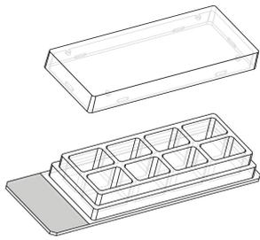
The 8 Well Chamber, removable is a removable silicone chamber, mounted on a glass slide, for cell culture and immunofluorescence stainings. It allows the use of standard cultivation, staining and mounting techniques with coverslip sealing. After mounting the glass slide with a coverslip, it is ready for the use with upright and inverted microscopes, as well as for long term storage. Suitable 24 mm×60 mm coverslips are provided by ibidi (10811).
