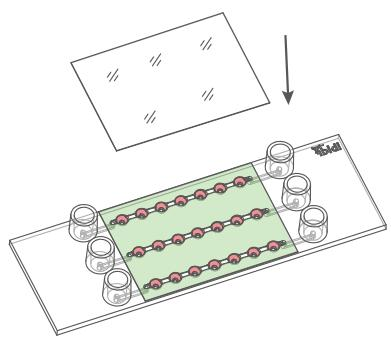
6. Incubate the slide for one hour at 37°C and 5% CO<sub>2</sub>.
