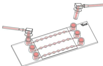
4. Open the clamped tubing and conduct your perfusion experiment.
