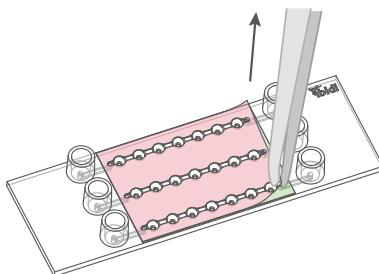
2. Remove the protective foil from the enclosed polymer coverslip and place it onto the adhesive part of the slide, ensuring a tight seal between them. Press down with your fingers to strengthen the connection.
