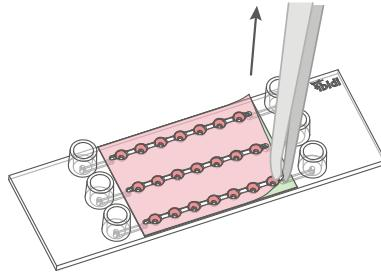
5. Remove the protective foil from the enclosed polymer coverslip and place it onto the adhesive part of the slide, ensuring a tight seal between them. Press down with your fingers to strengthen the connection.
