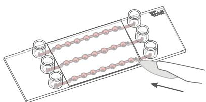
3. Grab the unsealed edge of the top coverslip and carefully remove it using strong tweezers.
