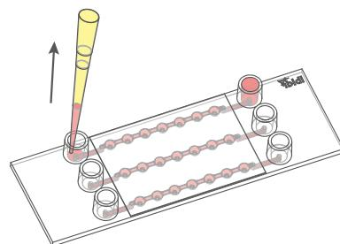
3. Fill 80 µl of fresh medium into one of the Luer ports, which will replace the channel volume by gravity flow.
