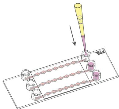
4. Slowly remove 80 µl from the opposite Luer port. If necessary, point the pipet tip inside the channel's inlet making a connection to the liquid inside the channel.
