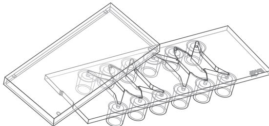
The sticky-Slide Tissue Engineering is the bottomless version of the  $\mu$ -Slide Tissue Engineering. It permits the mounting of a variety of bottom materials and is used for microfabrication applications and fluidic access.
