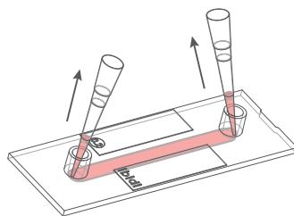
2. Slowly fill the respective channel volume of fresh medium into one of the reservoirs, which will replace the channel volume by gravity flow. Aspirate from the other reservoir by carefully using a pipet.
