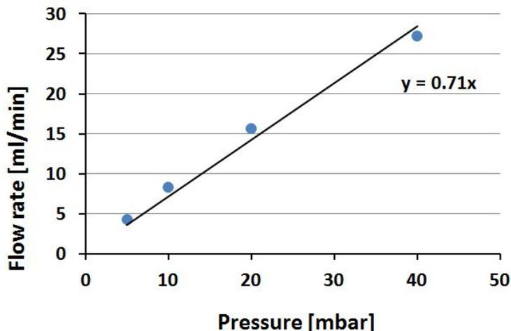
Figure 52: Example of a calibration curve showing the relation between flow rate and pressure.
