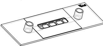
The  **$\mu$ -Slide I Luer 3D** is designed for perfusing a cell monolayer on a gel matrix.
