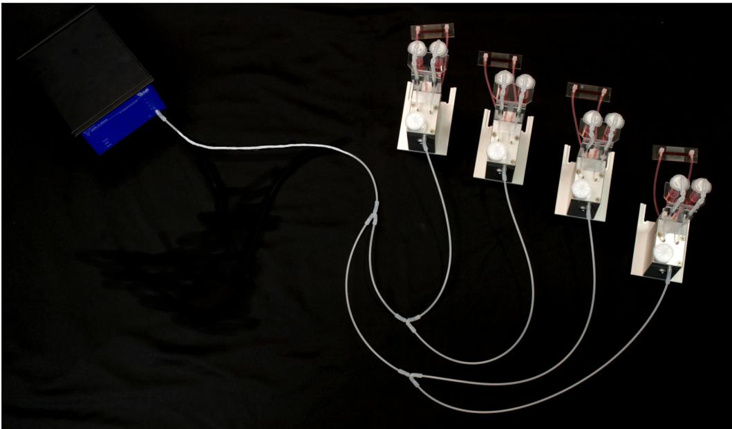
Figure 39: Connection of the ibidi Pump and four Fluidic Units via the Splitter Set for 4 Fluidic Units.
