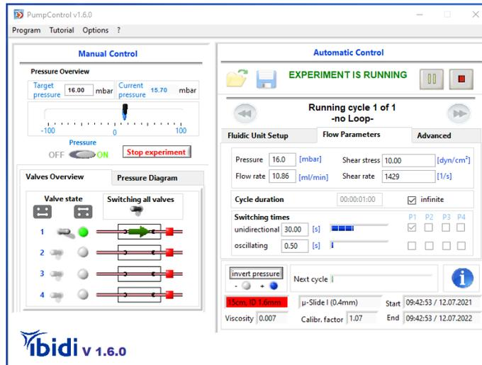
Figure 16: Main window of the PumpControl software
