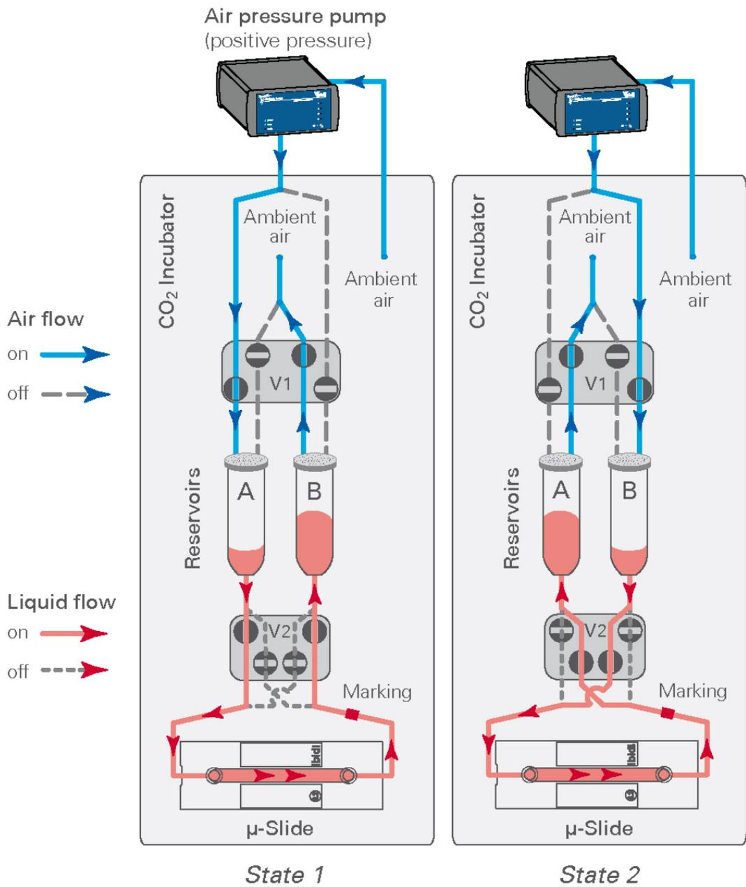
Figure 48: Working principle of the valves creating a unidirectional flow, using **positive pressure**.
