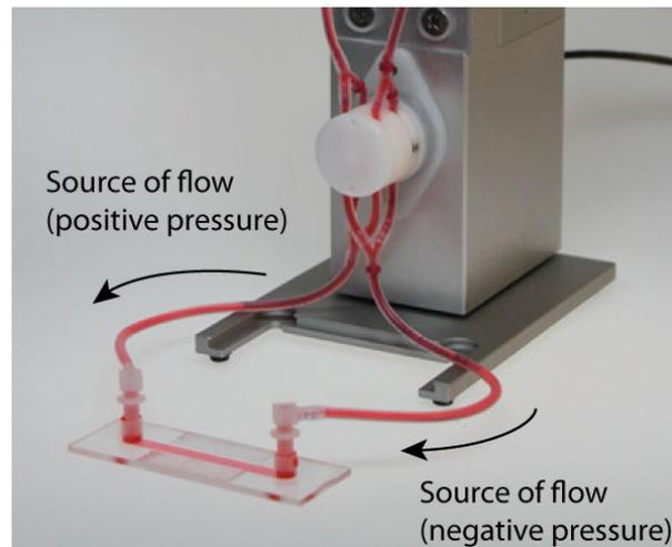
Figure 50: Flow direction with positive and negative pressure
