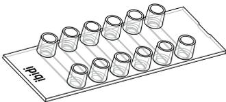
The  **$\mu$ -Slide VI<sup>0.4</sup>** provides six independent channels for general flow assays. It is also available as a glass bottom version (see [Table 8](#)).
