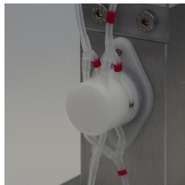
*Figure 24: Insert the tubing coming from reservoir A into the left side slots. The marked tubing goes in the rear slot.*
