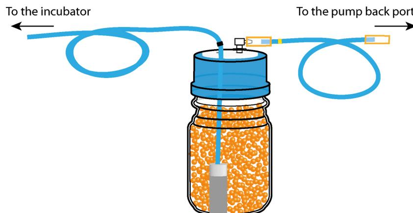
Figure 10: Assembled components of the Drying Bottle.
