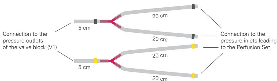
*Figure 40: Oscillatory Flow Kit for two Fluidic Units.*
