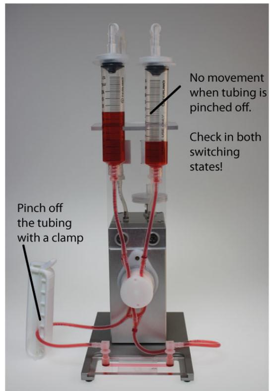
Figure 29: Pinch test for checking the correct insertion of the tubing into the valve.
