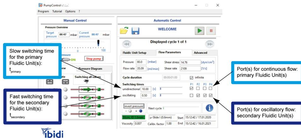
Figure 43: Settings of the PumpControl Software, when applying oscillatory flow to one primary and three secondary Fluidic Units. The ports P1 - P4 are the ports on the back of the Pump controller.
