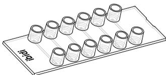
The  **$\mu$ -Slide VI<sup>0.1</sup>** provides six independent micro-channels for general flow assays.
