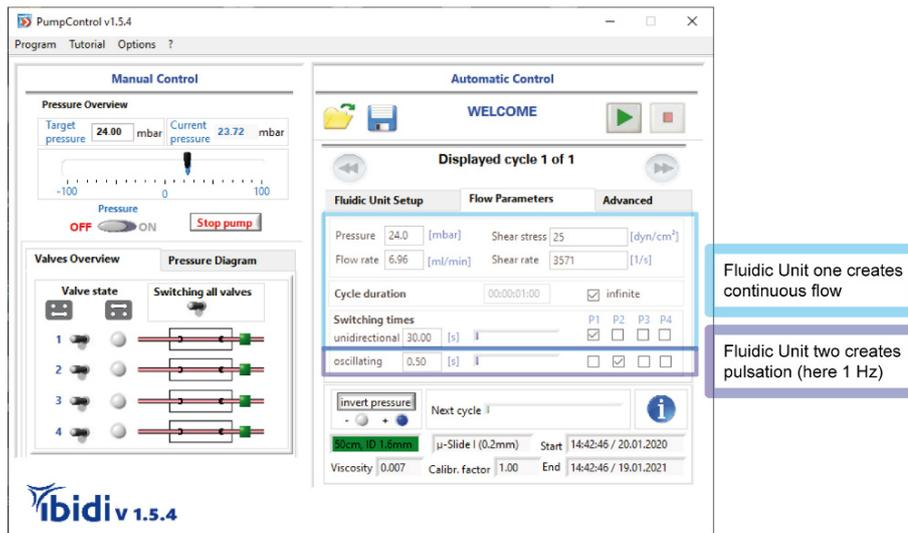
Figure 46: PumpControl example setting for pulsatile flow.
