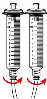
Figure 20: Screw the adapters tight into the reservoirs.
