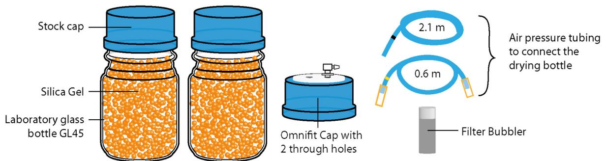
Figure 9: Components of the Drying Bottle setup.
