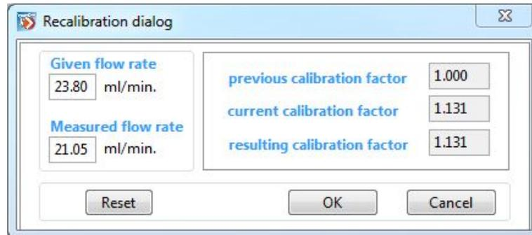
Figure 35: Recalibration dialog in the PumpControl software.
