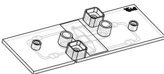
The  **$\mu$ -Slide ibiPore SiN** offers two crossing channels with a membrane separating the two medium reservoirs.
