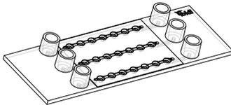
The  **$\mu$ -Slide Spheroid Perfusion** offers three channels with 7 small wells each, for the long-term cultivation and perfusion of 3D spheroids or organoids.
