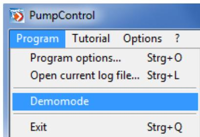
Figure 2: Changing from Demo mode to standard mode and back.
