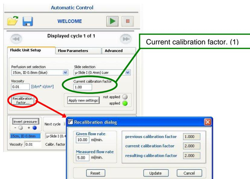
Figure 26: Recalibration Factor
