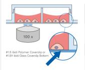
All ibidi µ-Labware products feature a thin Polymer or Glass Coverslip bottom, designed for cell culture with a specific focus on microscopy, offering exceptional image quality and cell adhesion.
