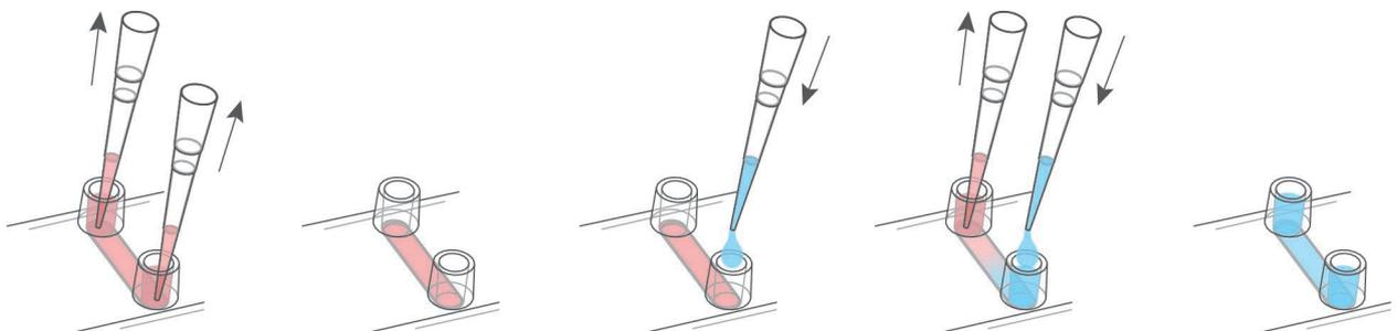
Continuous medium exchange with minimum three times the channel volume.
