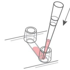
Filling a cell suspension into a channel of the  $\mu$ -Slide VI<sup>0.4</sup>.
