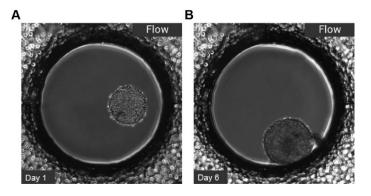
Figure 1: L929 fibroblasts show spheroid formation in the  $\mu$ -Slide Spheroid Perfusion. Examples of day 1 (A) and day 6 (B), perfusion with the ibidi Pump System, 0.74 ml/min. Phase contrast microscopy, 10x objective lens, well diameter 800  $\mu$ m.
