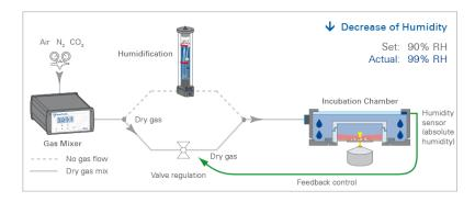
If the humidity is too high, condensation occurs. To decrease the humidity and prevent condensation, only dry gas enters the ibidi Stage Top Incubator.
