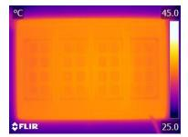
Stable and consistent temperature distribution in every well of a  $\mu$ -Dish  $^{35 \, mm, \, high}$ , a  $\mu$ -Slide 8 Well  $^{high}$ , and a  $\mu$ -Plate 96 Well Black in the ibidi Stage Top Incubation System. Images were acquired with a FLIR thermal camera. Please note that the pseudocolor scale in the multiwell image is slightly different.
