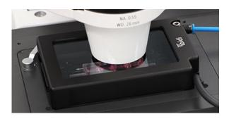
During a live cell imaging experiment, the evaporation in the stage top incubator should be kept as low as possible, underlining the need for a reliable humidity control. A constant and high level of humidity (>90% RH) in the stage top incubator is one of the keys to artifact-free results in live cell imaging.
