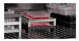
Cell culture vessels in the  $\mathrm{CO}_2$  incubator are usually cultivated in an open system, and are therefore in an equilibrium with the surrounding air. In standard  $\mathrm{CO}_2$  incubators, the humidity is created by evaporation from a water tray. Optimally, the relative humidity (RH) within an incubation system should be within the range of 90–95%.
