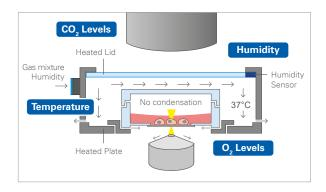
With fast and precise regulation of important environmental parameters, the ibidi Stage Top Incubators provide stable conditions for live cell imaging directly on the microscope.
