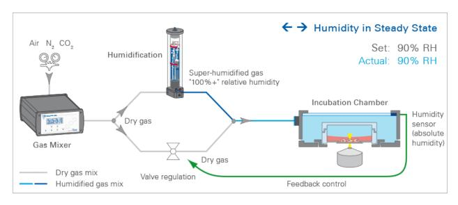
The ratio of dry gas and humidified gas is determined by the actual and preset humidity, and controlled by a feedback mechanism. In a steady-state system (e.g., when both the set and the actual RH are 90%), a mixture of humidified and dry gas enters the ibidi Stage Top Incubator.
