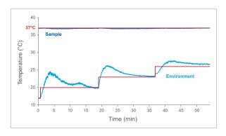
Sample temperature stability inside the ibidi Heating System Slide/Dish – Silver Line with Dish Holder and  $\mu$ -Dish  $^{35\,mm,\ high}$ , filled with cell culture medium (Sample). After equilibration of the sample inside the Heating System, the environment temperatures were increased stepwise (17°C  $\rightarrow$  20°C  $\rightarrow$  23°C  $\rightarrow$  26°C; max 27.7°C). The temperature of the sample inside the Heating System stably stayed at 36.9°C ( $\pm$  0.15°C).
