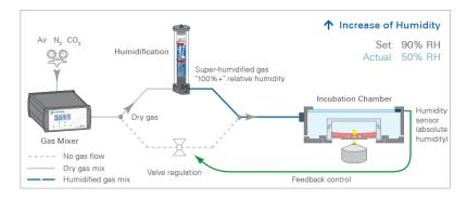
If the humidity is too low, evaporation occurs. To increase the humidity and prevent evaporation, only humidified gas from the humidification column enters the ibidi Stage Top Incubator.
